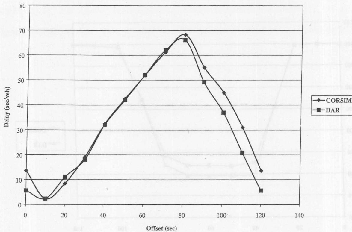
FIGURE 4 Comparison of arterial delay for a short link.
