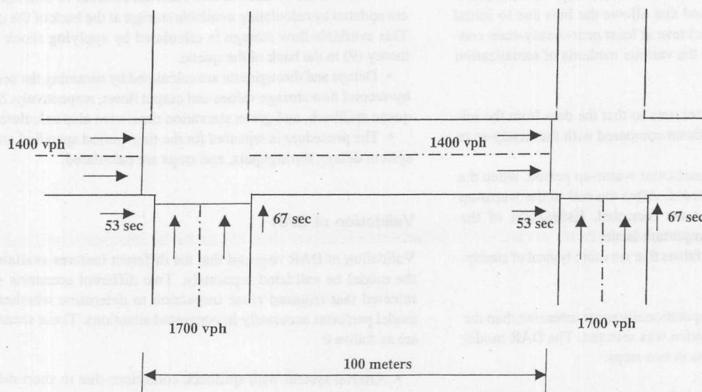
FIGURE 1 Arterial system with spillback conditions due to short downstream link (vph = vehicles per hour).
