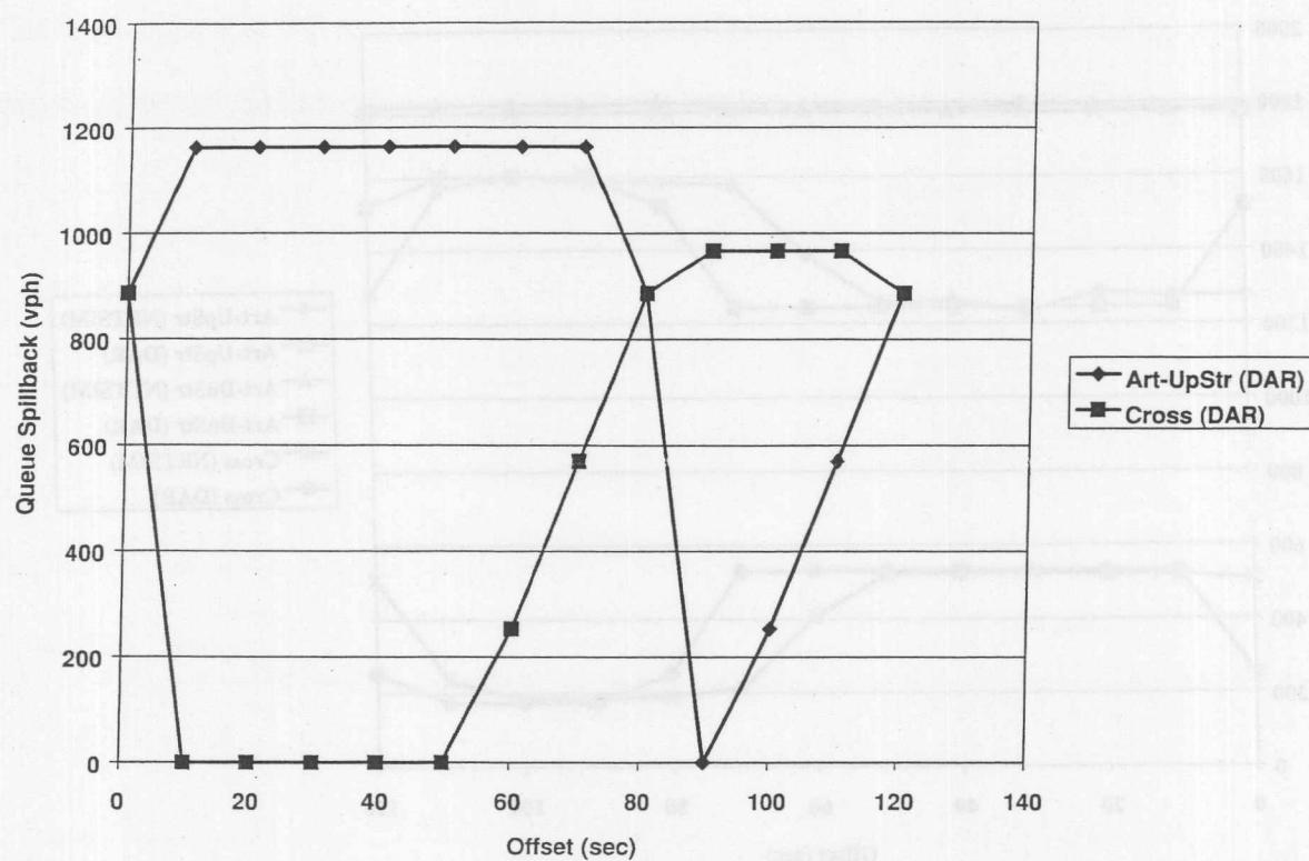
FIGURE 7 Modeling of spillback due to blocking of downstream link for an oversaturated link.
