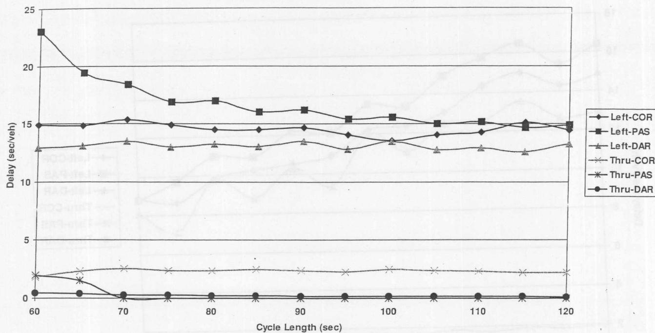
FIGURE 11 Comparison of DAR with PASSER III and CORSIM for TTI four-phase for 600 vphpl for 66-m (200-ft) link length.
