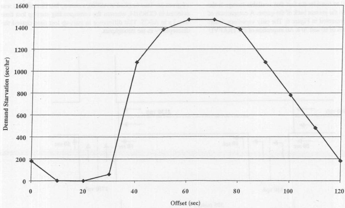
FIGURE 3 Demand starvation modeled at the downstream arterial movement for a short link in DAR.
