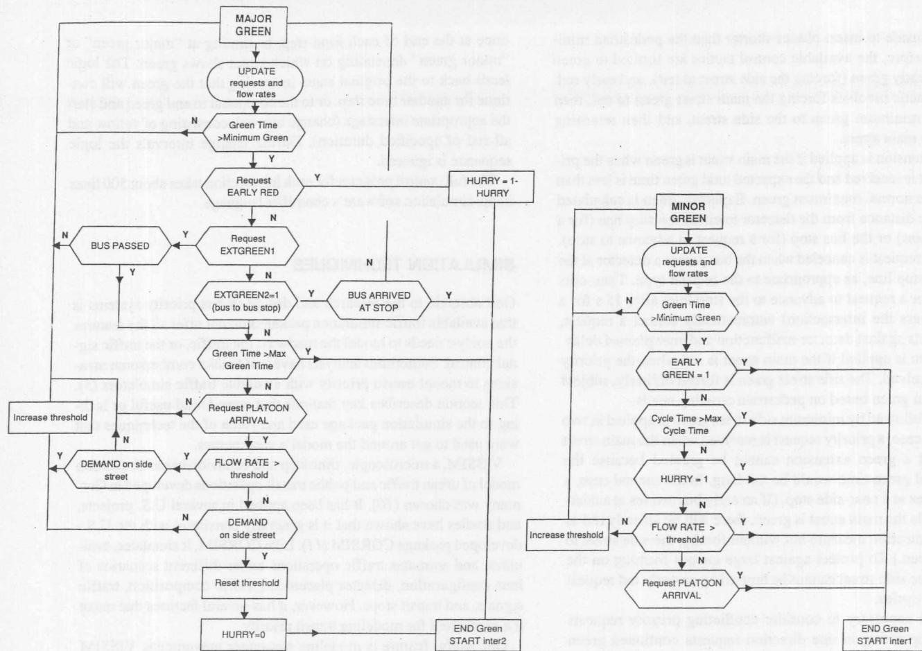
FIGURE 2 Traffic control logic.
