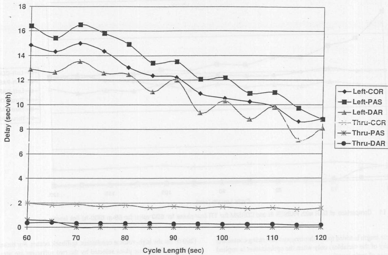
FIGURE 9 Comparison of DAR with PASSER III and CORSIM for TTI four-phase for 300 vphpl for 66-m (200-ft) link length.
