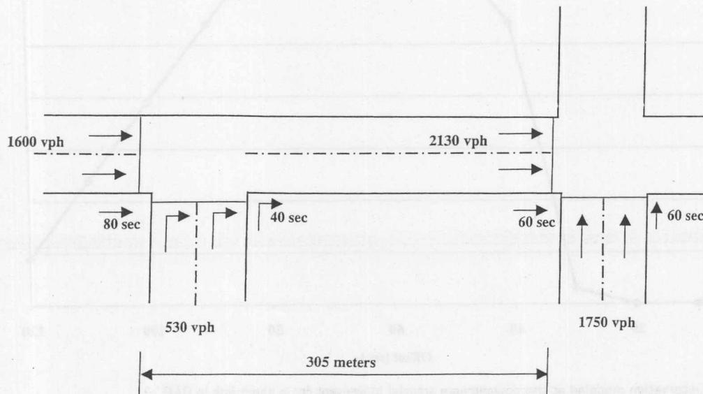
FIGURE 5 Arterial system with spillback conditions due to oversaturated downstream link.
